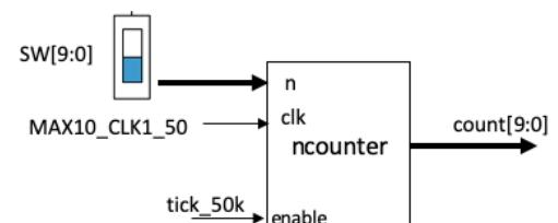
Modify **lab5task3** to include this new variable increment counter. Check that changing SW value changes the frequency.
