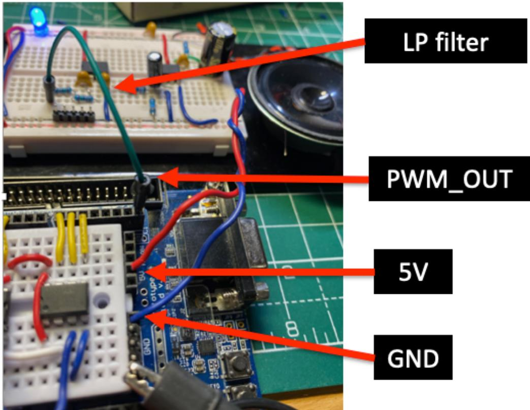
Measure the analogue voltage at the output of the LP filter with the scope or the multimeter for different value of SW. You should explore the full range of values by checking the follow SW[9:0] setting: 10'h3FF, 10'h200, 10'h100, 10'h80, 10'h40 etc. Why are these the correct values to explore?
