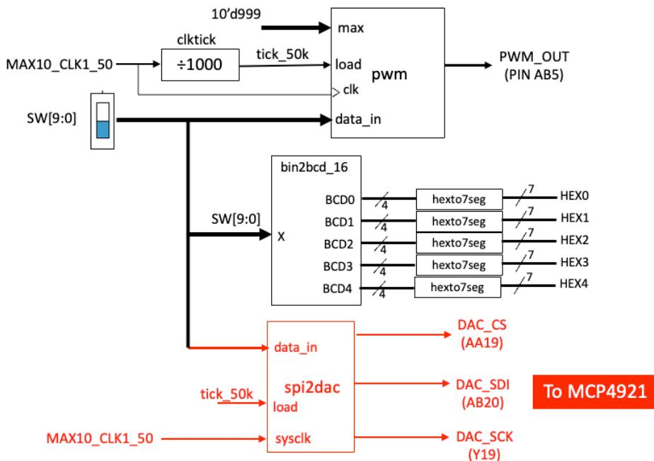
The **data\_in** value determined by the 10 switches (**SW[9:0]**) is loaded to the **spi2dac** module at a rate of 50k samples per second as governed by the **load** signal. The steps for this part are:
