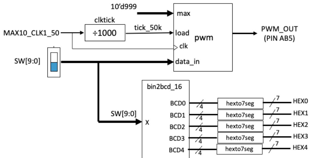
The **clk tick** module is used to provide a load pulse lasting for 1 clock cycle (20ns) with a period of 20us. This effectively determine the PWM sample frequency.
