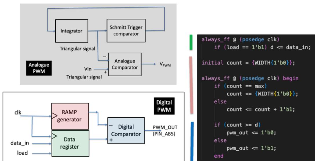
The analogue comparator is replaced with a digital comparator. The analogue input in Lab 2 is now replaced by a digital value **data\_in**, which is stored internally in the data register whenever load is asserted (high).
